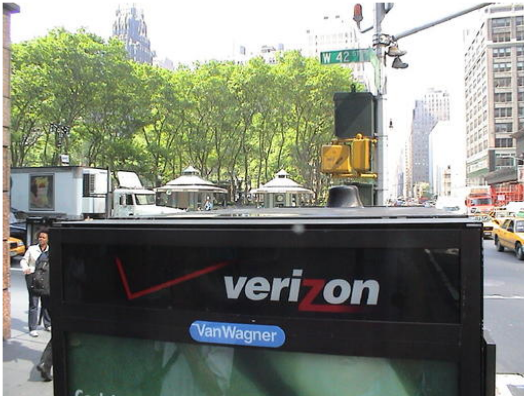
The black bump on this pay phone is a Wi-Fi antenna.
