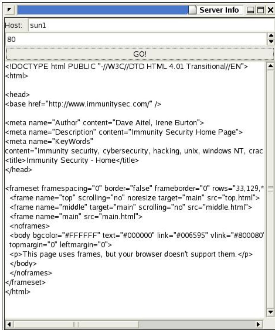
Figure 9. Clicking GO! loads the Web page and displays it in the TextView.
